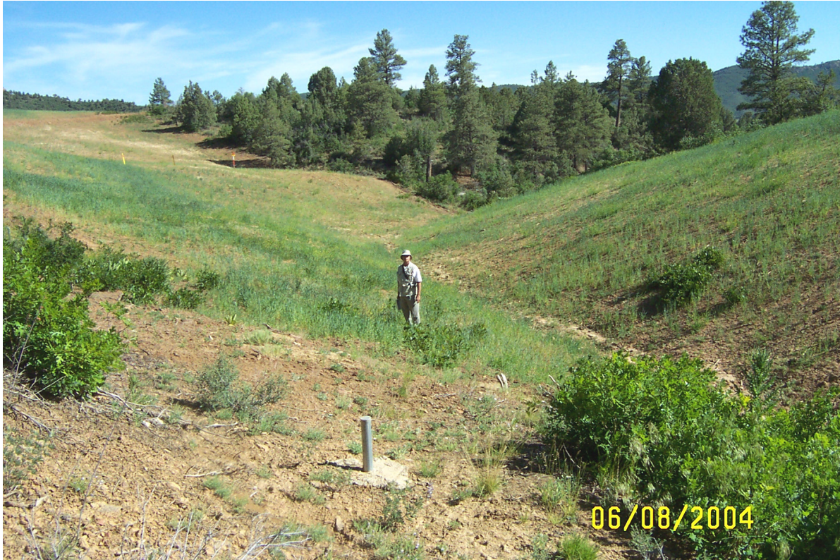
DUR 6/2004. PL-1. Inspector marks the location of missing boundary monument BM-6; the north witness corner is in the foreground.
